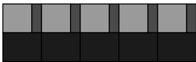
Figure 3. For short compute intensive operations, the prefetch operation may not complete as fast as the previous processor task. In this event the processor may still stall waiting for data from memory, but the length of the stall is shortened.
