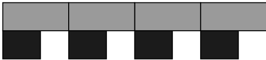
Figure 2. Prefetch operations issued in advance of a compute intensive phase bring data into cache before processor completes previous task. This eliminates a processor stall to wait for data from memory.
